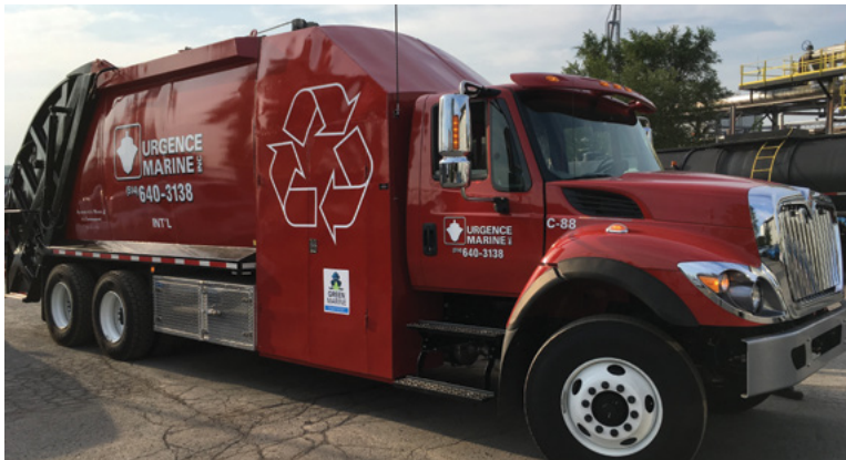
An Urgence Marine’s truck is equipped with separate compartments for oily waste, galley waste, medical waste, pyrotechnics and other specific recyclables.
